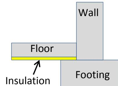
The barrier that the ants had to breach was a 2 foot wide by 18 inches deep concrete **Footing** that was laid around the perimeter of the house. A 11 inch thick continuous concrete **Wall** was poured on top the footings with a dome concrete ceiling. A 1/8 insulating material was laid down before the 4" floating concrete **Floor** was poured in order to keep the floor from getting cold in winter time.
